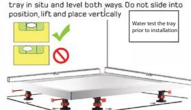
$oldsymbol{6}$  . Refer to step B of the waste instructions. Fix all legs to the floor, screw fix legs where possible. Fix the centre leg last to form a stabalising point.
